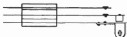
SW-1-C MAKE SWITCH (SMALL CONTACTS)
