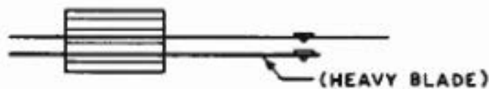
SW. 1-Z1 MAKE SWITCH (SMALL CONTACTS)
