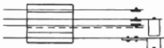
SW-30C MAKE-BREAK SW. (LARGE CONTACTS)
